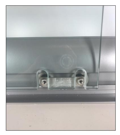
On View Series Frameless Sliding Glass Doors there is a horseshoe shaped cutout at the bottom of the door. A Carriage assembly will be installed in that location. To install the Carriages, repeat the installation process used for the top of the door.
