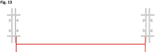
Stud Spacing for a 48" Wide Panel: Stud Spacing Width = 48 1/8" \*\*Measurement Location Shown Above\*\*
